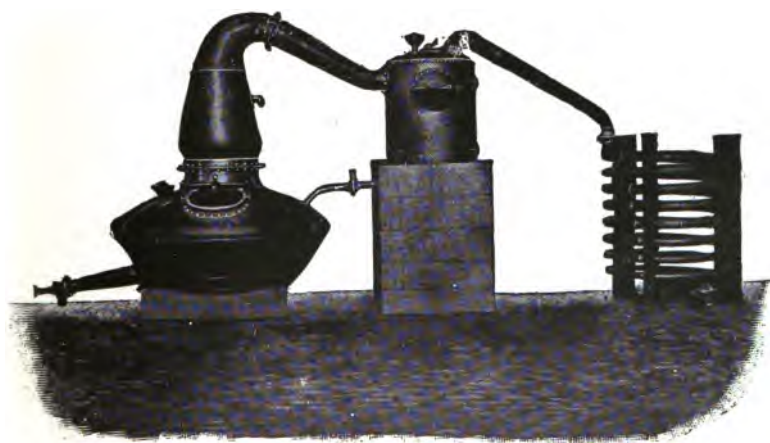
FIG. 35. POT STILL, WITH RETORT AND CONDENSER. (Messrs. Blair, Campbell & McLean, Ltd., Glasgow.)
